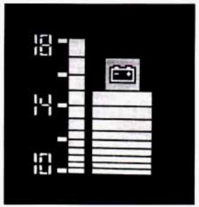
The red charging system light is on the bottom driver's-side corner of your standard cluster. It is part of the digital cluster voltmeter.
